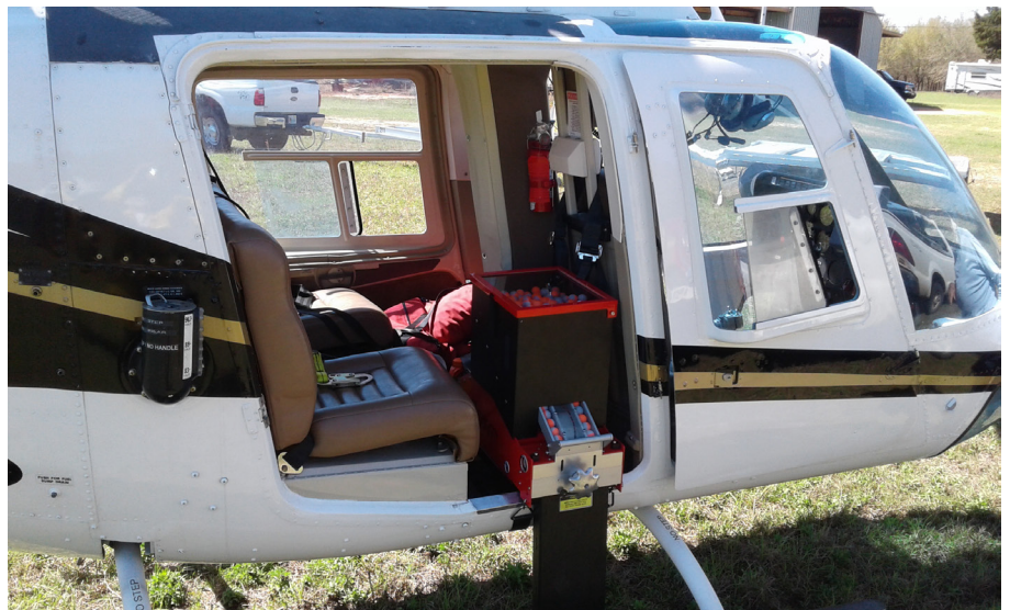
Helicopter used to ignite the prescribed burn using a Red Dragon Aerial Ignition Device at the Yellow River Water Management area in Santa Rosa County, Florida. Credit: Steve Brown, Northwest Florida Water Management District
