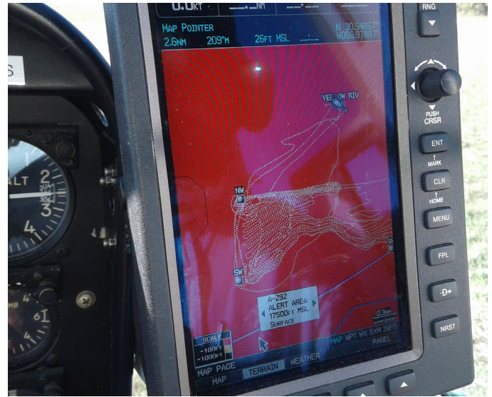
Helicopter GPS displays where ignition balls were dropped. Credit: Steve Brown, Northwest Florida Water Management District
